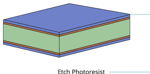
**Place Artwork:** Artwork patterns from the customer (circuits and land patterns) are placed on the film coated surfaces of the core. Each surface has its own artwork pattern.
