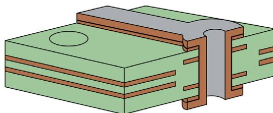
**Strip Resist:** Developed dry film resist is chemically removed. Tents that were placed have prevented plating from occurring in “non-plated” holes.
