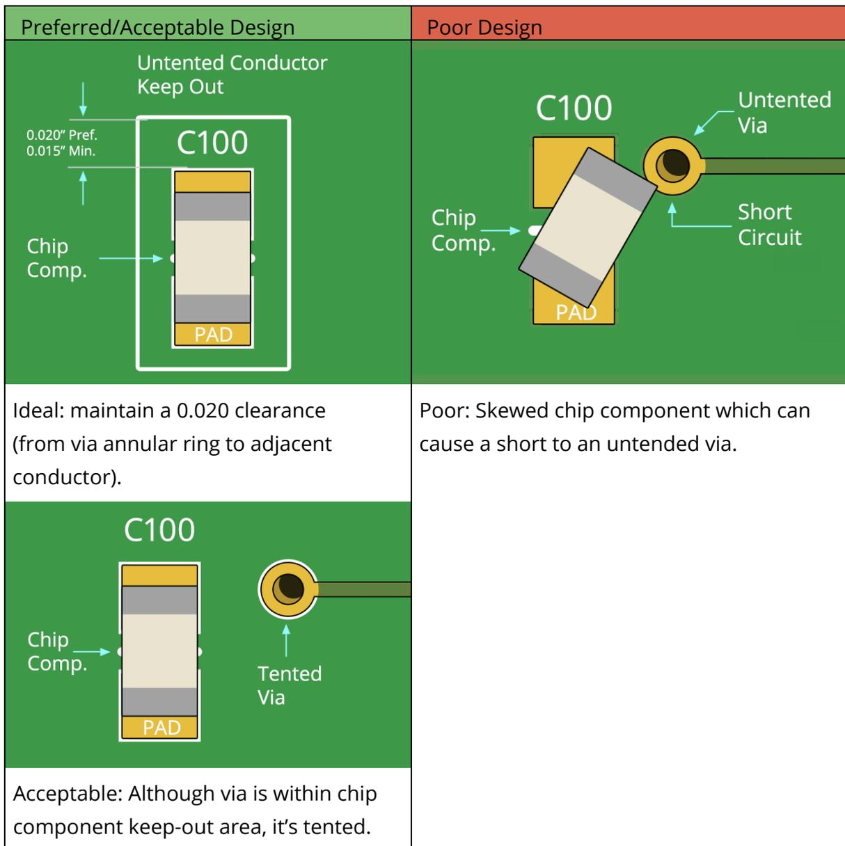
Figure 16 - Via Placement Guidelines Near Chip Components
