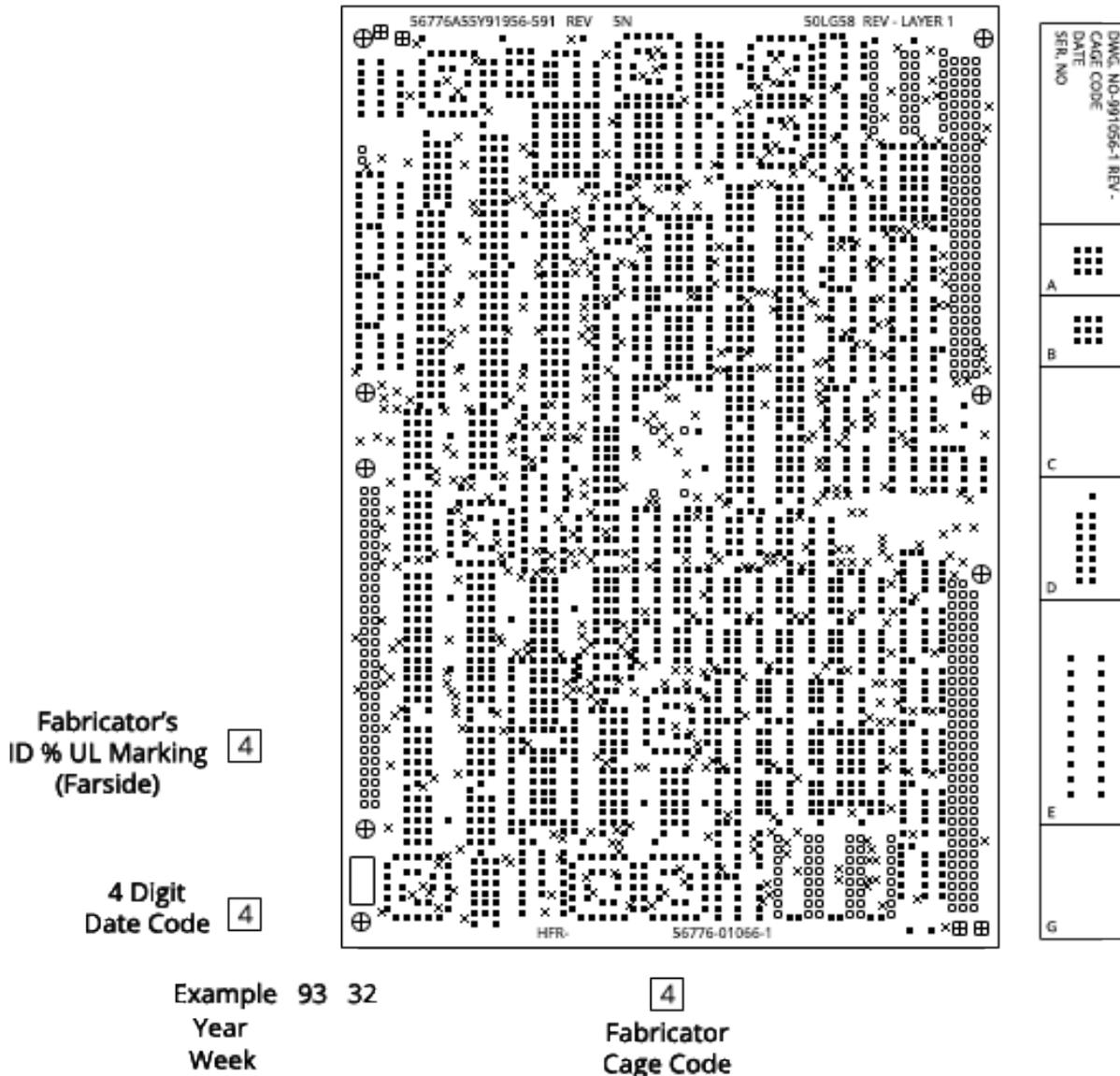
Figure 73 - Drill Pattern on a PCB
