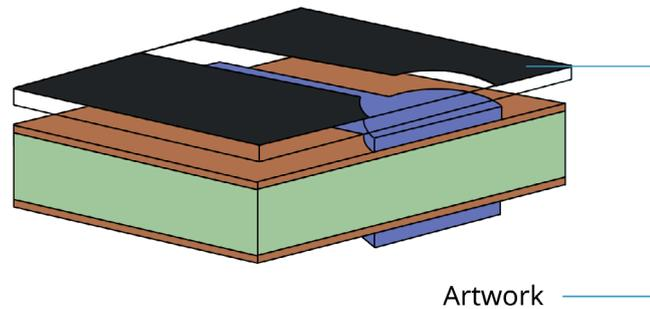
**Etch:** To chemically remove copper from core in all areas not covered by film resist, which creates a discrete copper pattern.
