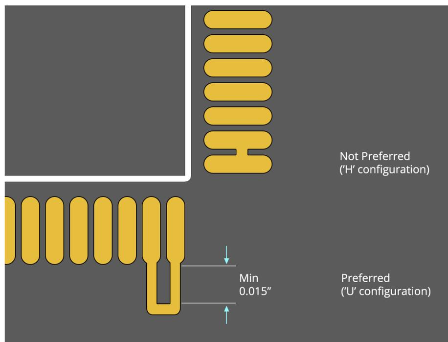
Figure 27 - “U” Configuration for Routing Leaded SMD Components
