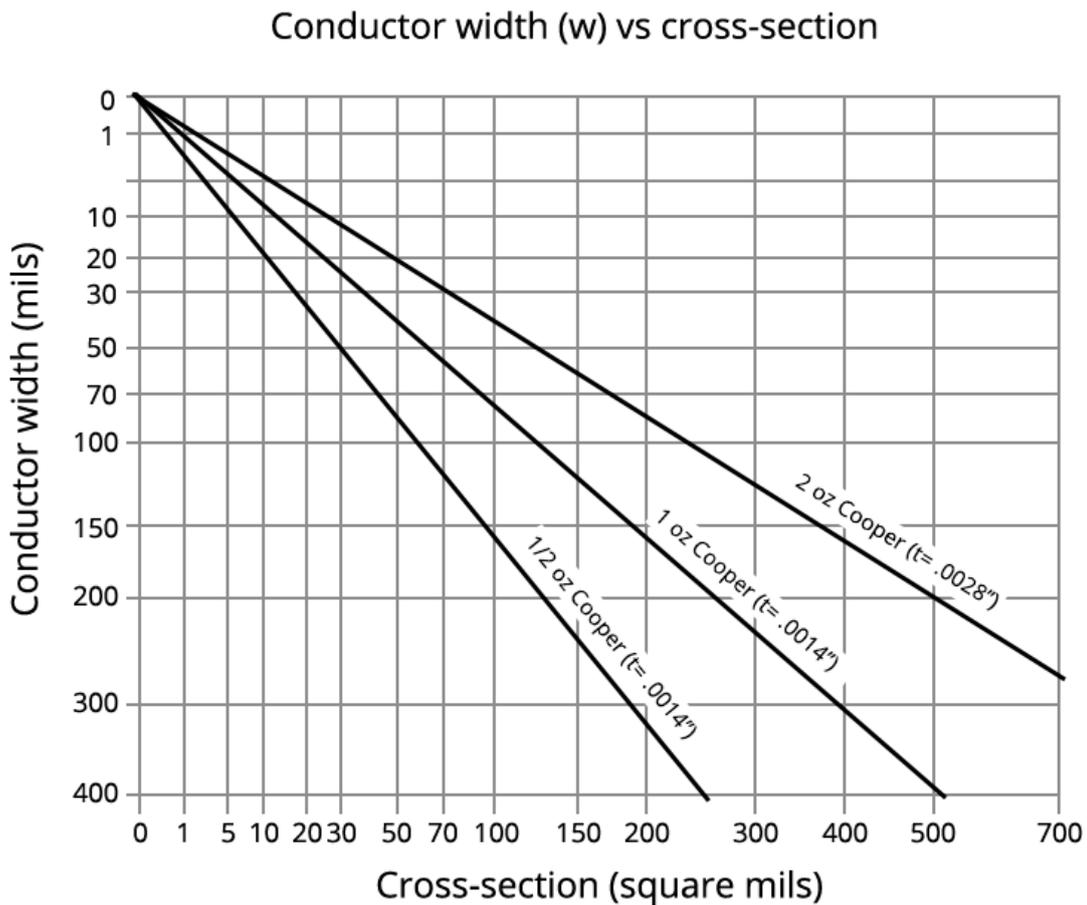
Figure 7 - Encapsulated Conductor Widths<sup>[2-10]</sup>
