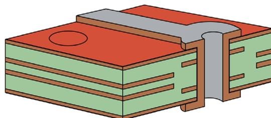
**Solder Mask and Cure:** Liquid photoimageable mask is applied to each surface and dried to the touch. Artwork is also applied and exposed. PPanel is developed, leaving mask pattern defined by artwork.
