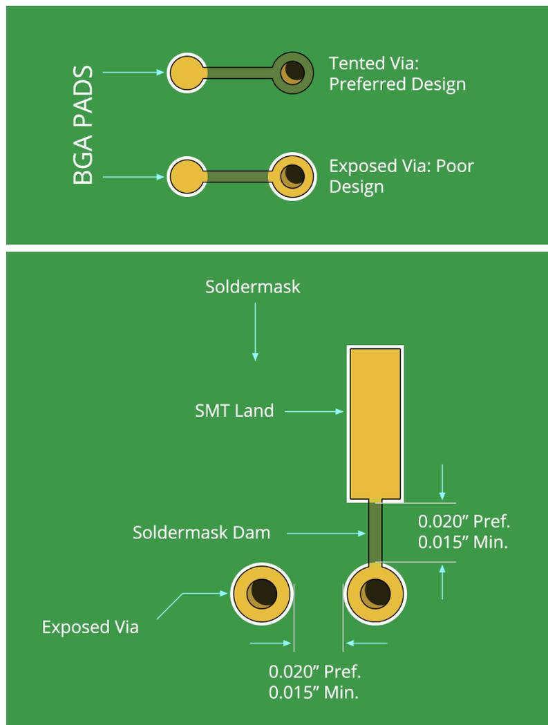
Figure 14 - Recommended Via Tenting Applications on a BGA
