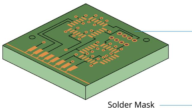
**Hot Air Solder Leveling (most common PCB surface finish):** Panels processed through a molten solder bath, which covers all exposed copper surfaces.
