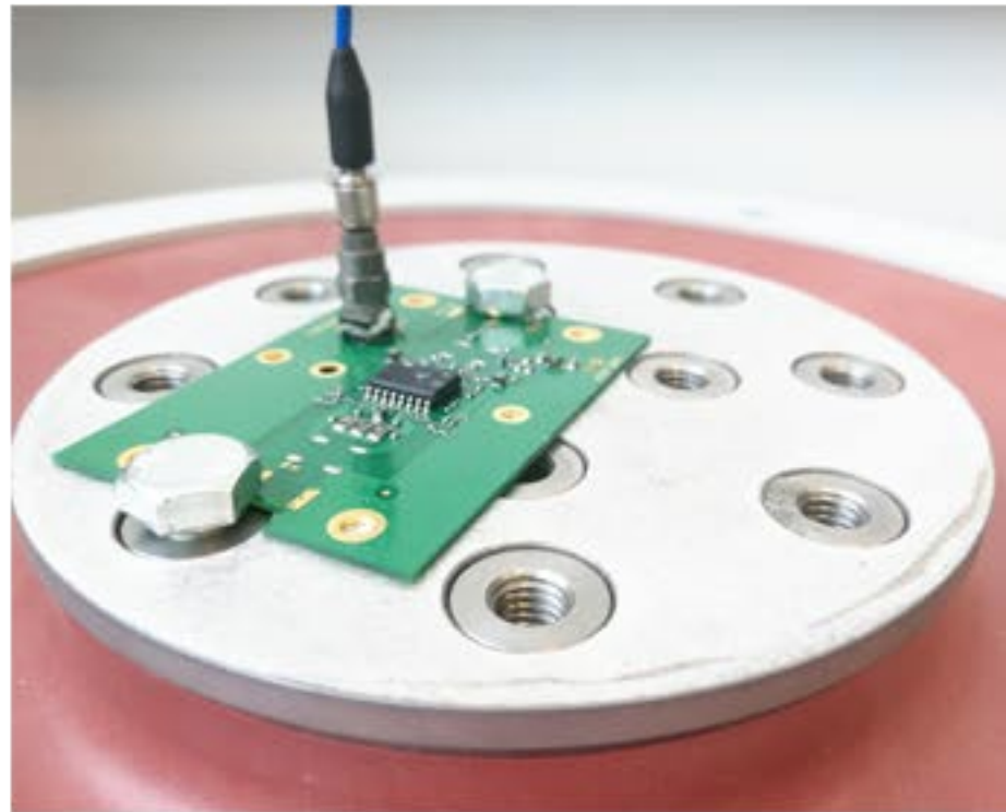
This image shows a test fixture being used for vibration testing in a finished board.
