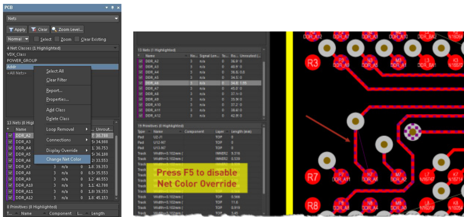
Fig. 19.6 - Setting for the highlighting color for net objects in the PCB panel
