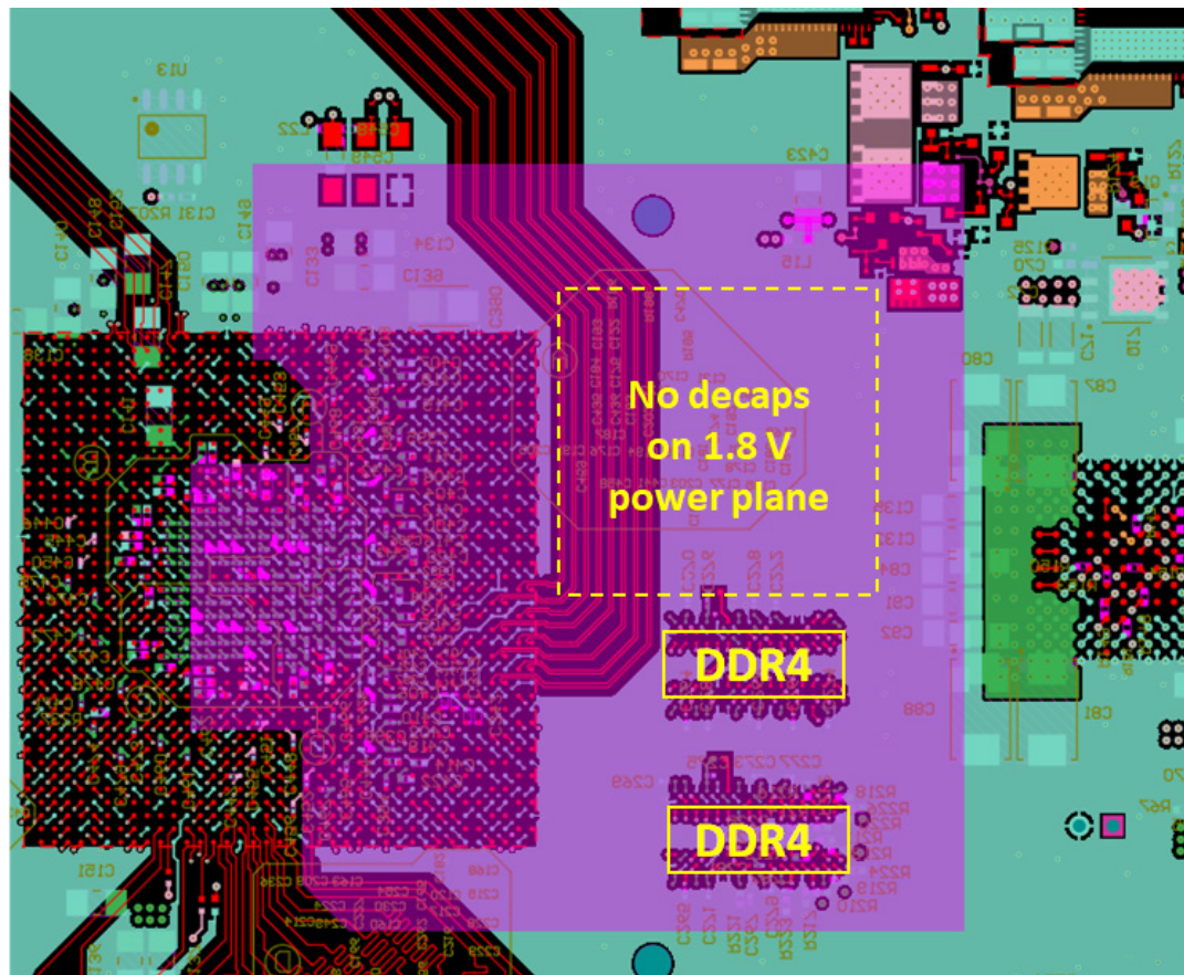
Figure 1: PLL_1V8 net flagged by missing decoupling capacitors.
