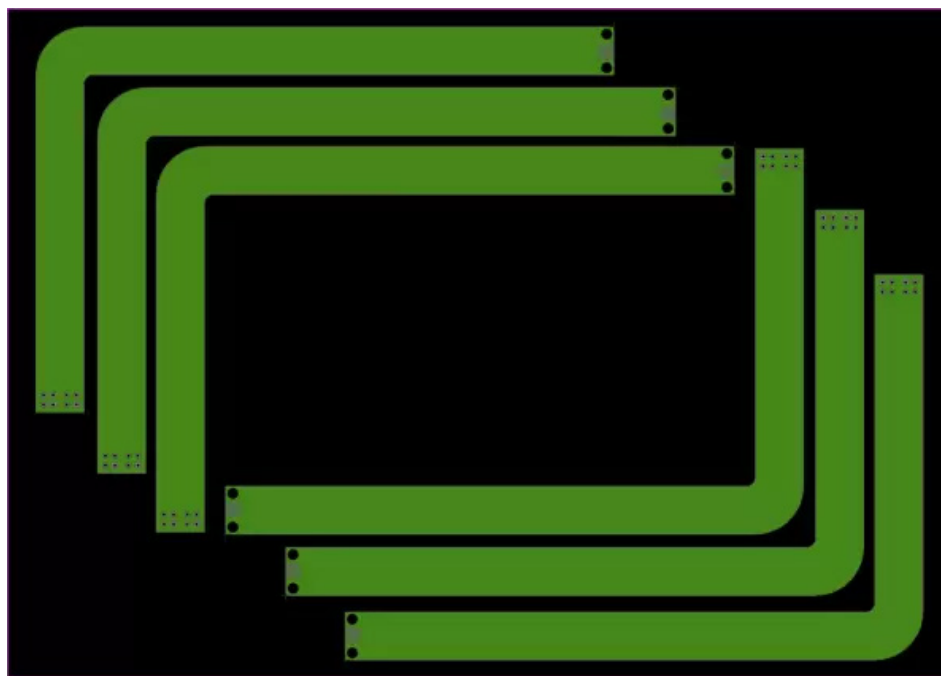
Embedded Board Array panelization of the CNC gantry flex circuit.
