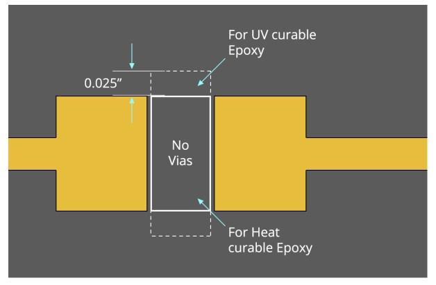
Figure 20 - Via Clearance Guidelines for Wave Soldering
