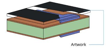
**Etch:** To chemically remove copper from core in all areas not covered by film resist, which creates a discrete copper pattern.
