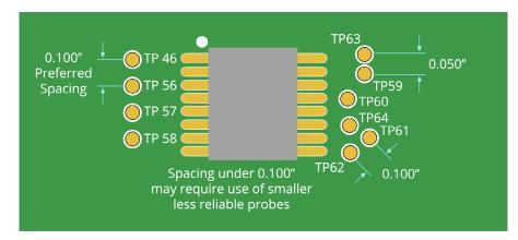
Figure 42 - Test Pad Spacing
