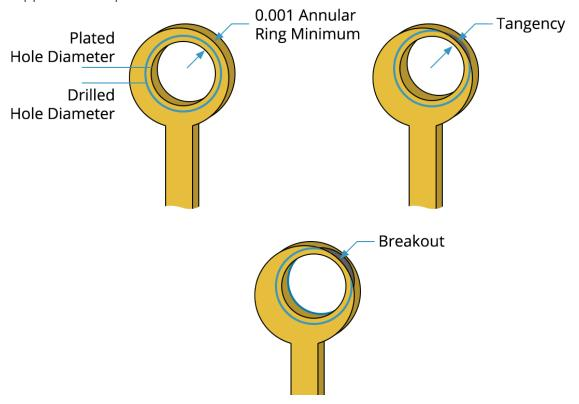
Figure 13 - Drilled and Plated Hole Diameters
