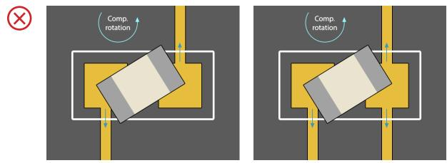
Figure 26 - Connecting Traces to Component Lands When Using Soldermask
