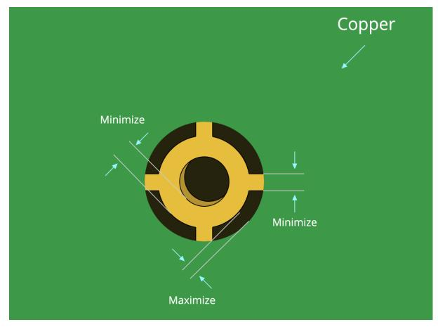
Figure 29 - Typical Thermal Relief Pattern
