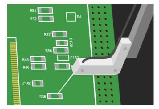
Figure 84 - Floating Probe
