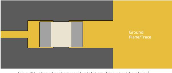
Figure 24b - Connecting Component Lands to Large Conductors (Poor Design)
