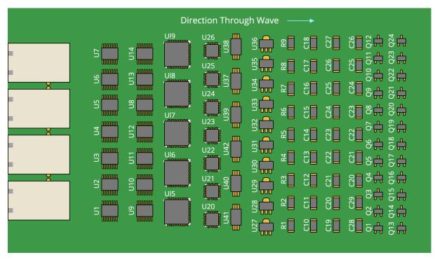
Figure 32a - Clustering Large components Requires High Temp Reflow (can damage Chips)
