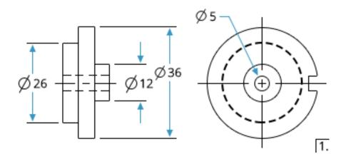
Figure 69 - Dimensioning Holes from a Side View
