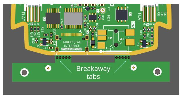
Figure 49 - Breakaway Tabs
