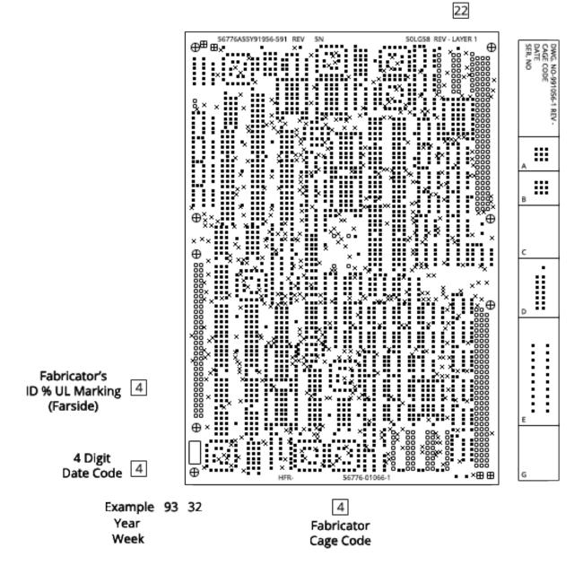
Figure 73 - Drill Pattern on a PCB
