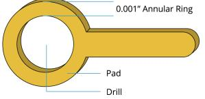
Figure 12 - Recommended Annular Ring Width
