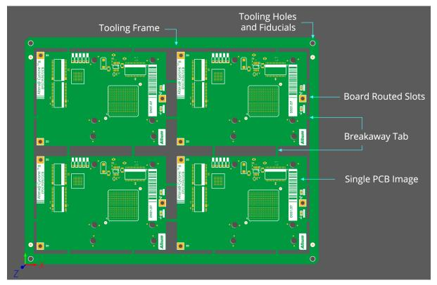
Figure 45 - Rectangular Circuits in a Single Panel with Tooling Holes and Breakout Tabs
