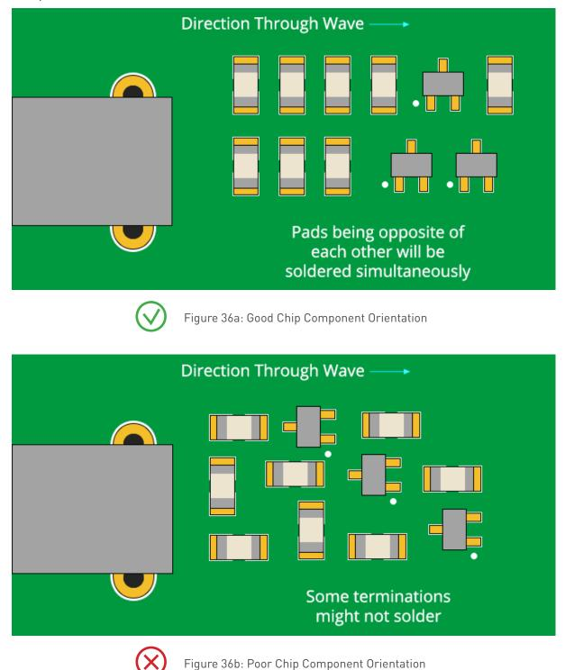
The more shadowing of smaller components you have on your board from the solder wave, the more likely your PCB will end up with open solder joints. Ensure that the soldering direction of your board is positioned in a way that large components will not shadow the smaller chip components as shown in Figure 37 below.
