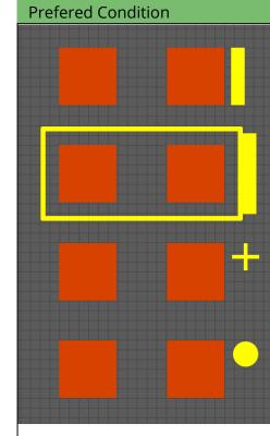
Unmarked polarized locations can complicate the assembly process, which can lead to delays to process the first article. Not to mention the danger associated with mounting a polarized capacitor in reversed orientation.
