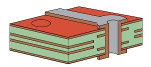
**Solder Mask and Cure:** Liquid photoimageable mask is applied to each surface and dried to the touch. Artwork is also applied and exposed. PPanel is developed, leaving mask pattern defined by artwork.
