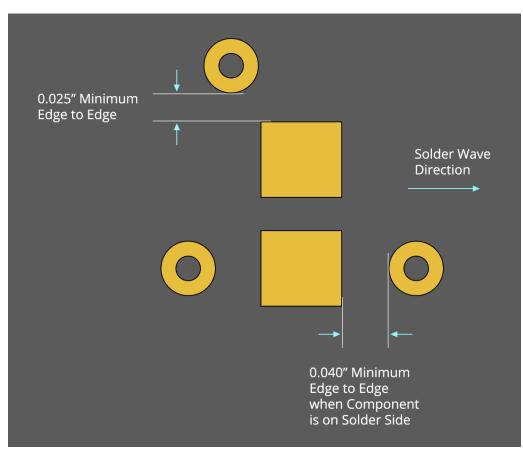
Figure 22 - Via Component Spacing for Wave Soldering
