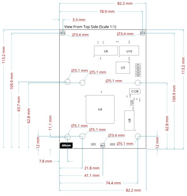
Figure 68 - ADD Well Dimensioned PCB
