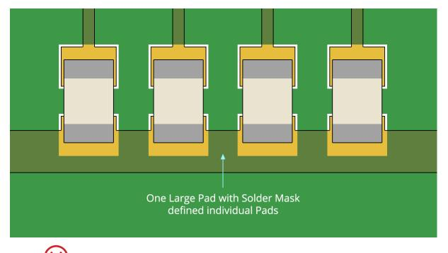
Figure 25c - Connecting Pads of Closely Spaced Components (Poor Design)
