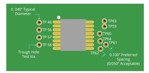
Figure 41 - Through-hole Test Via
