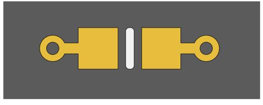
Figure 21b - Not Recommended Connections of Vias to Pad Components (Poor Design)
