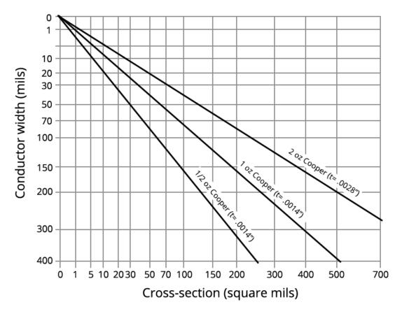
Figure 7 - Encapsulated Conductor Widths<sup>[2-10]</sup>
