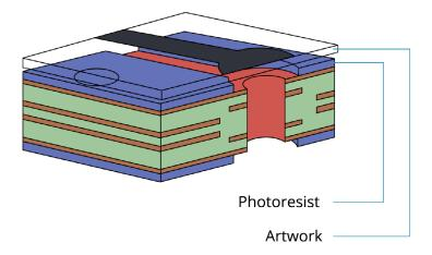
**Copper Pattern Plate (electroplating):** Additional copper (as well as tin) is electrically plated into the exposed electroless copper surfaces, as well as tin.
