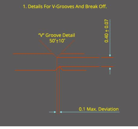
Figure 51b - Required Grooving Lines and Details on V Grooved Panel
