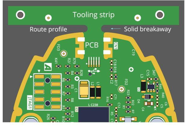
Figure 50 - Solid Breakout Pip
