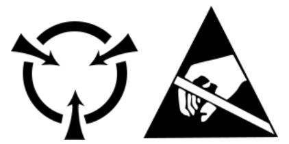
Figure 80 - Electrostatic Discharge Markings
