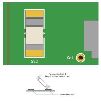
Figure 33: Termination Pulled Away from Component Pad Due to Poor Thermal Balance (Tombstoning)
