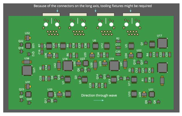
Figure 35b: Bottom Side Component Orientation for Wave Solder (Non-Preferred)
