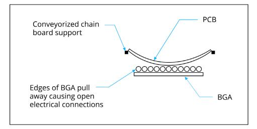
Figure 38 - Example of the Bow-and-Twist Effect on BGA Devices
