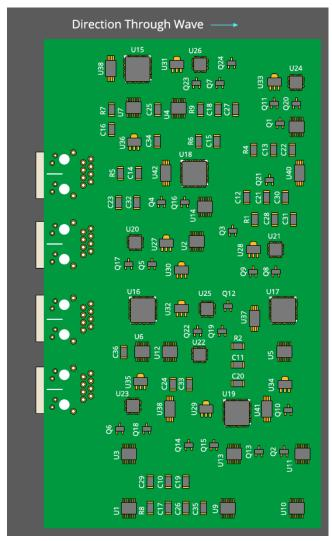
Figure 34 - Unpreferred Board-to-Solder Orientation
