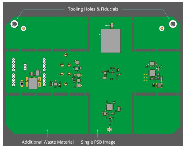
Figure 52 - Irregular Board with Infill Panels
