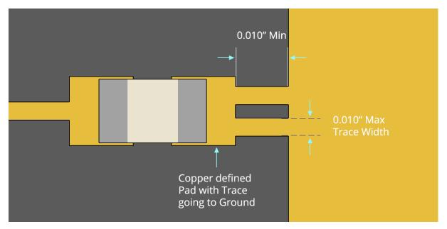
Figure 24a - Connecting Component Lands to Large Conductors (Good Design)
