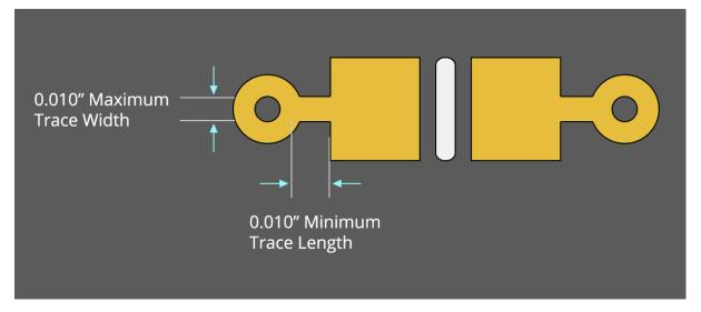
Figure 21a - Recommended Connections of Vias to Pad Components (Good Design)
