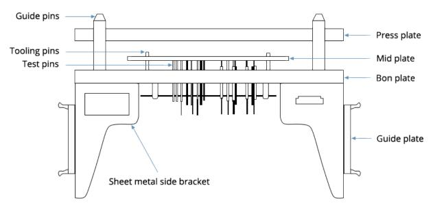
Figure 83 shows an example setup for a bed of nails tester.
