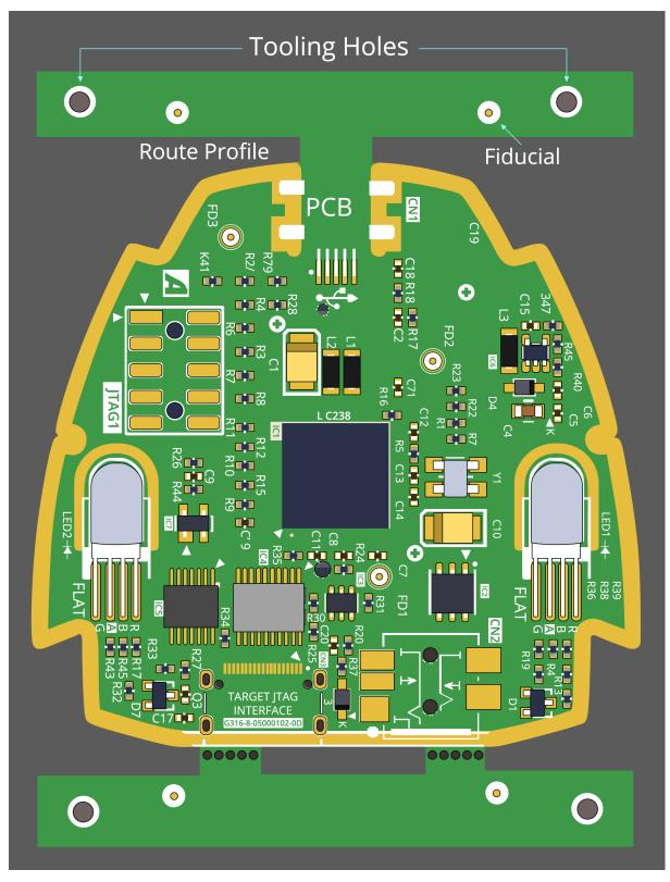
Figure 48 - Proper Tooling Hole Placement on a PCB
