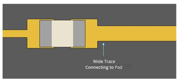
Figure 23b - Connecting Large Traces to Component Lands (Good Design)
