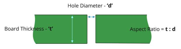
Figure 18 - Determining an Aspect Ratio for a PCB
