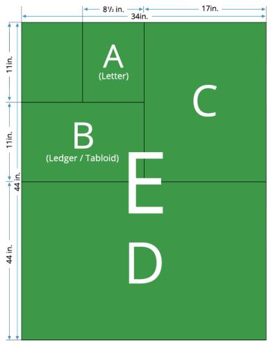
Figure 53 - Standard Drawing Sizes for PCB Documentation
