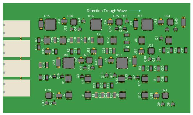
Figure 32b - Spreading Out Large Components for Better Thermal Distribution
