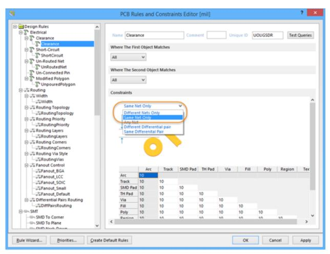
*Figure 1: Setting clearance values in the PCB Rules and Constraints Editor.*
