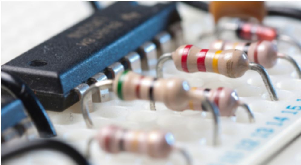
A circuit built on a breadboard for testing
