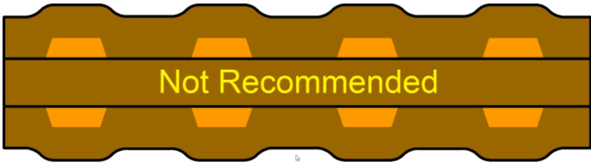
Figure 7: Adjacent-layer copper traces are not recommended.
