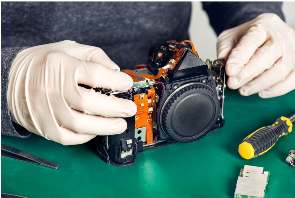
Digital cameras are already using lots of flexible PCBs.
