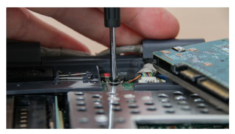
Make sure your can has enough clearance for the components it's shielding.
