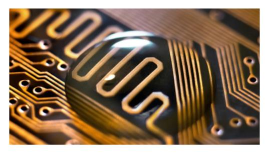
High speed designs will include many new design techniques including measured trace lengths
