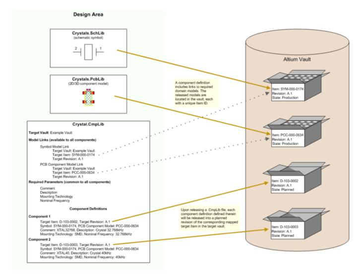
Definition of a component. All data required for a component is specified on the design-side within a dedicated Component Library file, including links to the lower-level released domain models and parametric information.
